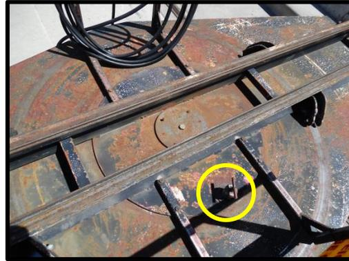
Spring loaded keeper pin, holds table in position, pull pin to turn table. Load MUST be balanced to the center of the table.
