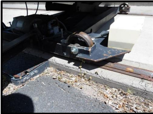
Carriage wheels run on angle iron rail, 56 in from top of angle to top of angle. Crisp Yard lifts have 36 inch wheelbase, should be larger.
