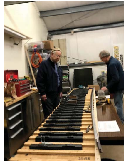
Greg Slobodzian, left, explains how to build curved track panels to Ken Olsen and Doug Wilkenson
